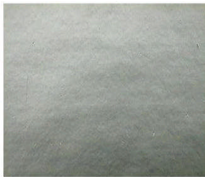
2 K Solvent-Borne Acrylic Urethane Coating 0.51 w t% B Y K 3 2 0 0.053 w t% PolyFox PF-656
