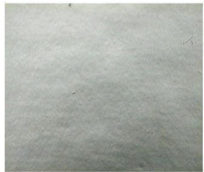
2 K Solvent-Borne Acrylic Urethane Coating 0.51 w t% B Y K 3 2 0 0.053 w t% PolyFox PF-6320
